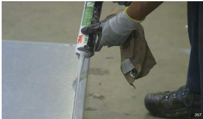
3M™ Polyurethane Sealant 740 moisture cures to a flexible seal/bond between exterior skins and metal framework and between wood flooring and metal framework. Tensile strength up to 580 psi is enough to replace mechanical fasteners in many situations.
